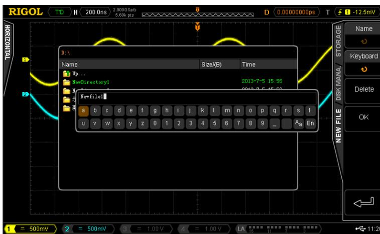
This oscilloscope supports Chinese/English input method. The filename or folder name can contain letters, numbers, underscores, spaces and Chinese characters and the length of the characters is limited to 31 bytes (one Chinese character occupies two bytes). Please input the desired name to create a new file or folder by referring to “**English Input Method**” and “**Chinese Input Method**”
