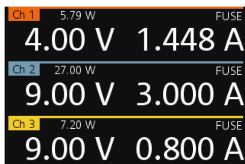
Figure 5-11: Fuse switched on for the respective channel
