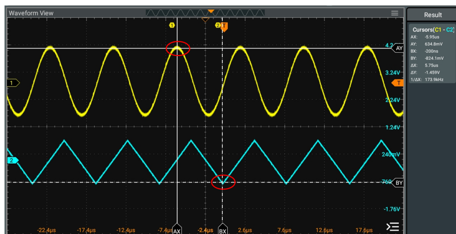
Figure 10.9 Track Measurement (before Horizontal Expansion)
