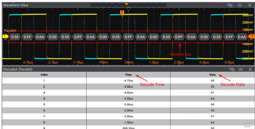
Figure 19.3 Parallel Decoding Event Table
