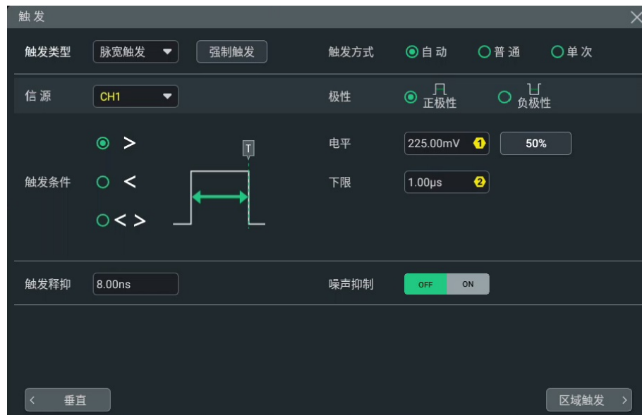
Figure 8.5 Pulse Trigger Setting Menu
