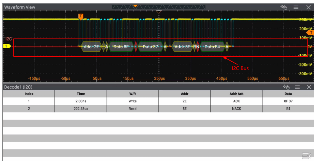
Figure 19.9 I2C Decoding Event Table
