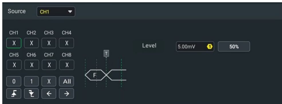
Figure 8.11 Pattern Trigger Setting Menu of DHO Series 8-CH Model
