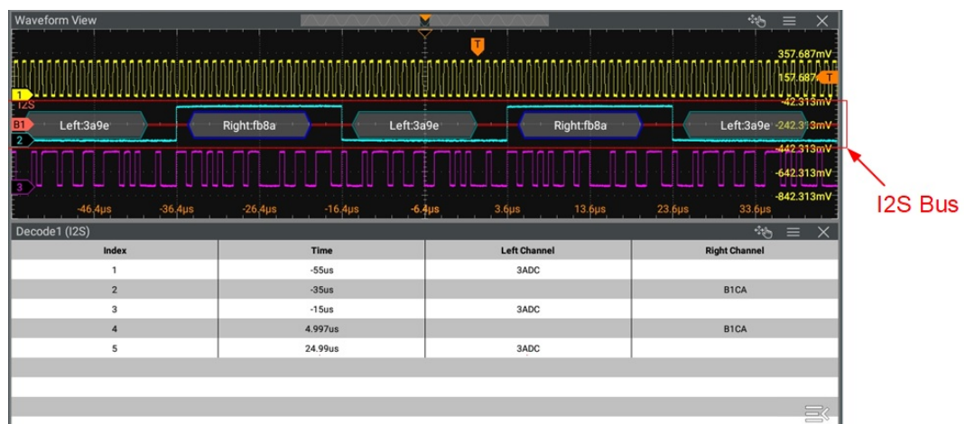
Figure 19.19 I2S Decoding Event Table
