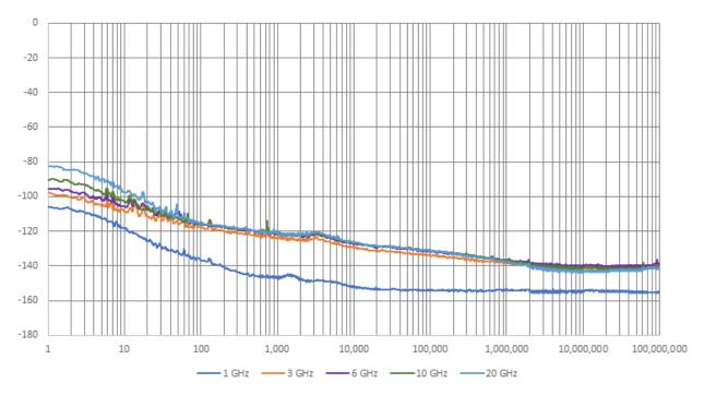
Figure 6: Measured residual phase noise using the external LO mode for the N5194A.
