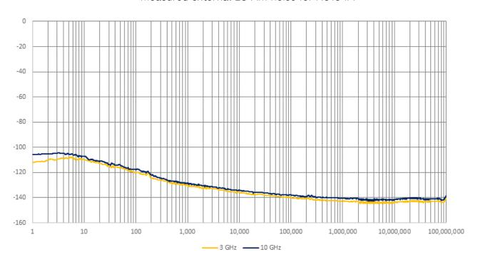
Figure 8. Measured AM noise using the external LO mode for the N5194A.
