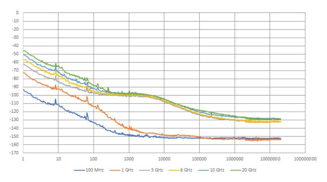
Figure 9: Measured absolute phase noise using the external LO mode for N5192A.
