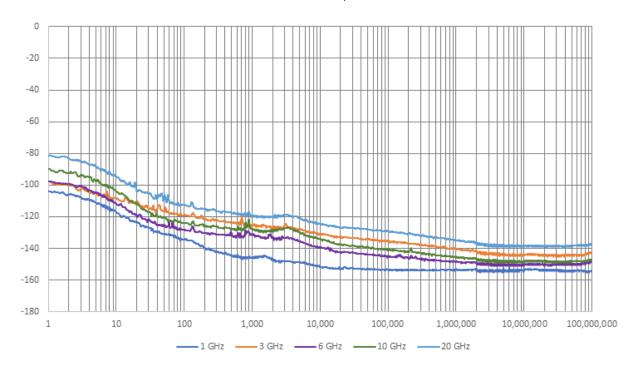
Figure 5: Measured residual phase noise using the internal LO mode for the N5194A.
