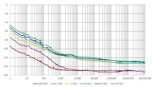
Figure 4. Measured absolute phase noise using the external LO mode for the N5194A.
