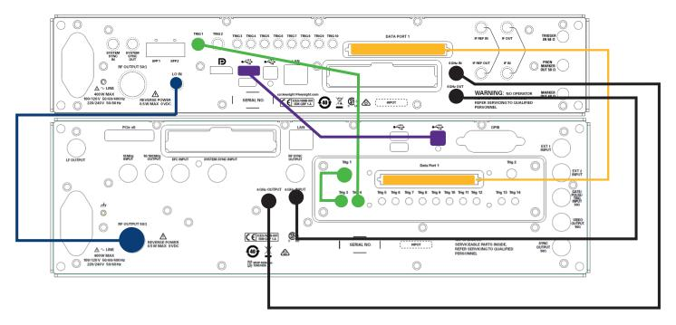
Figure 14. Connections between the UXG agile vector adapter and the UXG agile signal generator.
