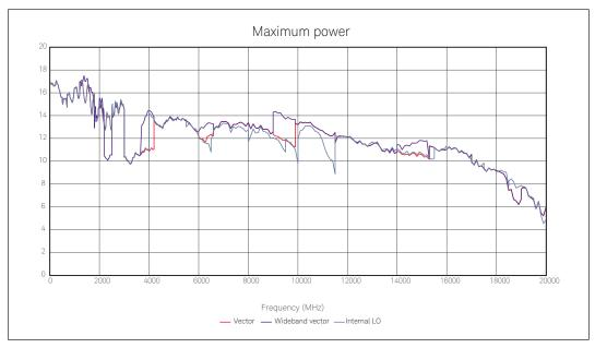
Figure 2. Maximum CW power (measured)
