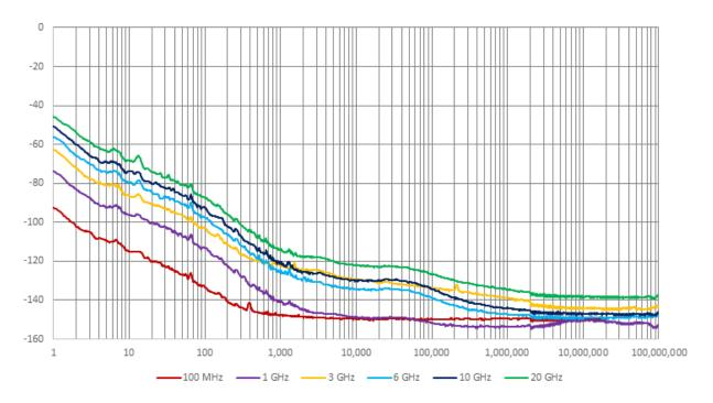
Figure 3. Measured absolute phase noise using the internal LO mode for the N5194A.
