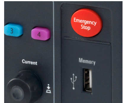
Figure 12. The emergency stop button shuts down all outputs immediately.
