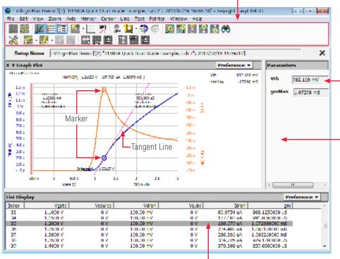
Parameters pane displays the parameters extracted by user functions. They can be displayed in the graph pain for graph image export
