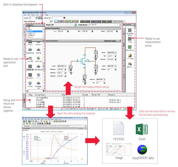
Main screen provides easy access to the data in the workspace and measurement capabilities
