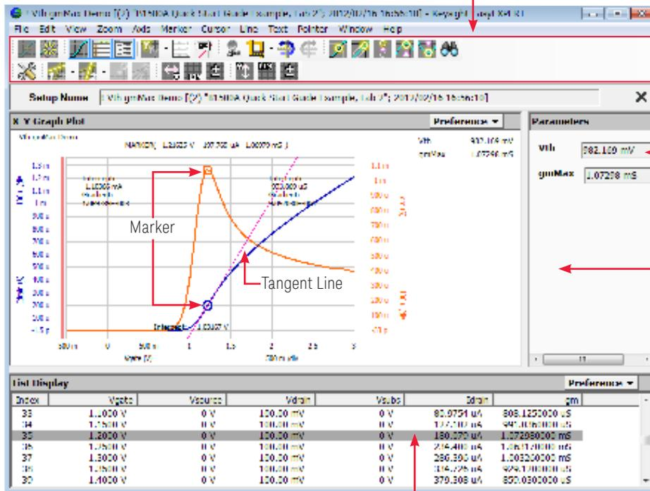
Parameters pane displays the parameters extracted by user functions. They can be displayed in the graph pane for graph image export
