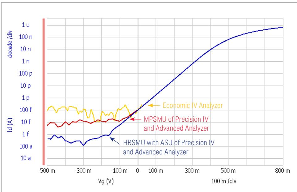
Transistor measurement example across multiple levels from sub-pA that is measured by different SMUs.
