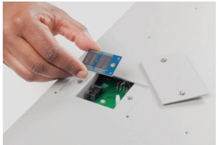
Figure 8. Installing the N7908A BBR hardware option on an APS power supply
