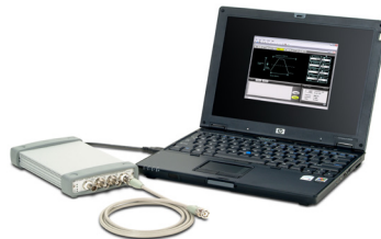
U2761A used as a standalone instrument
