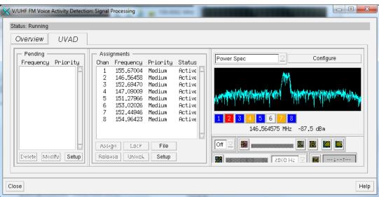
With Release 4.1.0 of Signal Surveyor 4D, users will have more direct control over the Digital Down Converters and the option to purchase multiple DDC's (using option N6841A-MFP). This option will provide up to eight DDC's with bandwidths up to 200 kHz.
