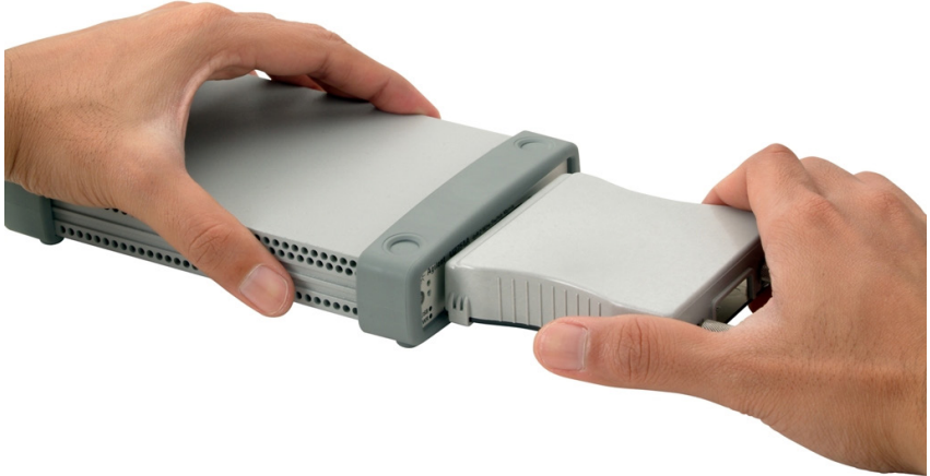
Figure 1. U2922A with U2751A used as a standalone device
