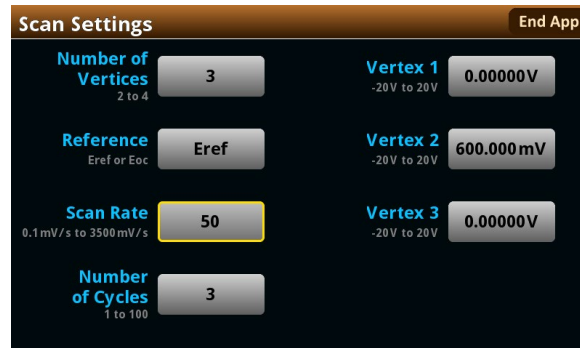
2450-EC Cyclic Voltammetry Test Configuration Screen
