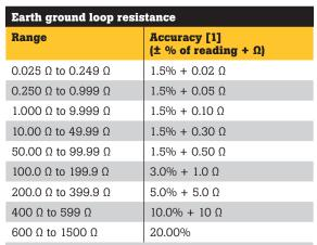
[1] Loop resistance with no inductance, conductor centered and perpendicular to jaw.
