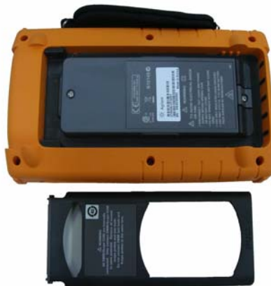
Figure 8-2 Disassemble the stand from the instrument
