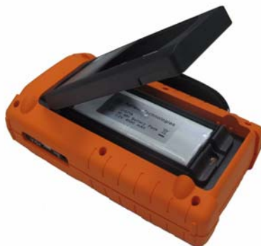
Figure 8-5 Remove battery pack cover without removing stand
