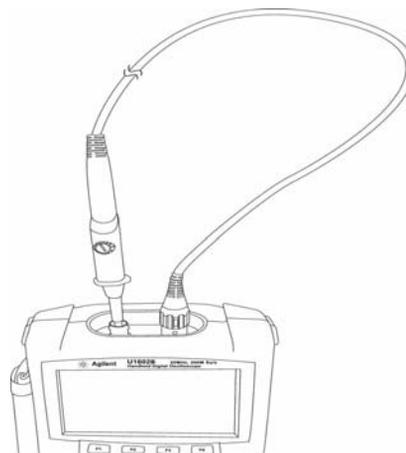
Ensure the shape of the displayed pulse is properly compensated. If not, adjust the trimmer capacitor to obtain the flattest square wave possible.
