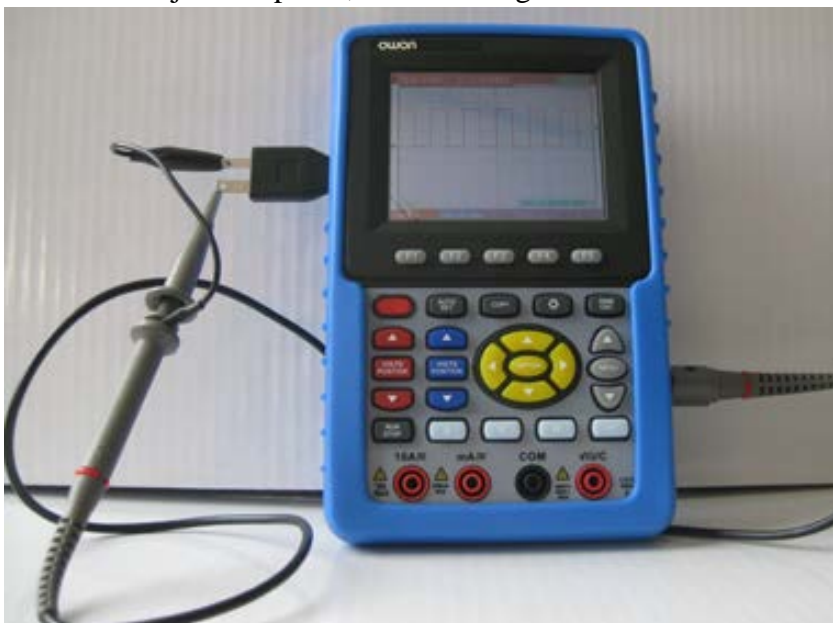
Fig.3. The connection of Square-wave test signal
