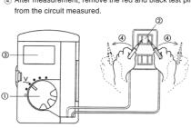
This instrument employs the average measurement system and some error is made to the display of waveforms other than sine waves. The accuracy guaranteed frequency range is 45 Hz to
